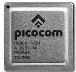
Picocom PC802 5G Small Cell PHY SoC
